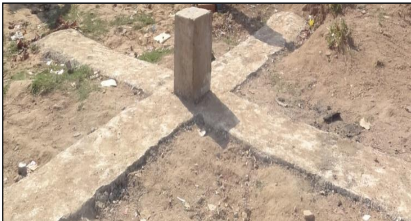
Figure 11: Pillar of Primary Control Point located in Gwalior District
