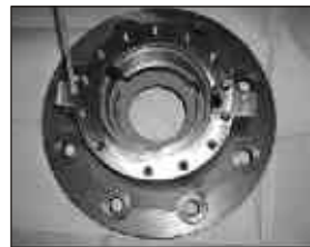
Fig 18 - Modified Pinion Carrier
