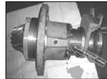
Fig 11- (A) Oil leakage at cut-out portion
